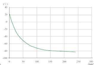
When cabinet running at -80°C, open the lid and put in a 1.5ml minitype test tube (water injected)
